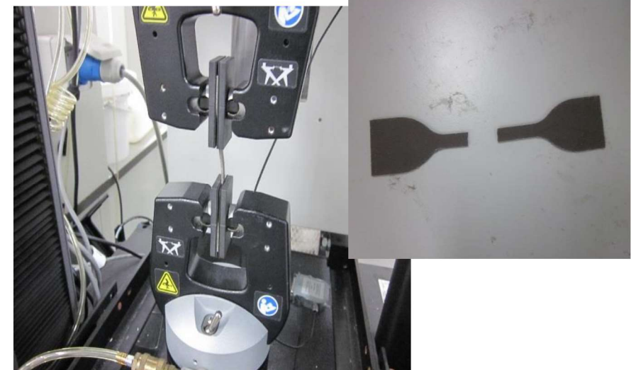
3. Put the stripe on the clamp and control the grip length with 60mm, and gauge length with 25mm.
